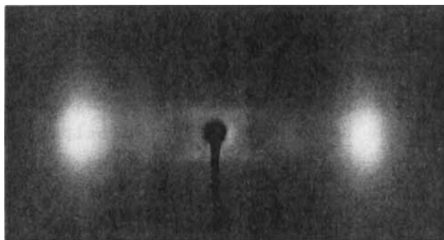
Fig. 1. DDA-9 ( n = 10 ) polyester, T_{NI} = 123.6^{\circ}\text{C} , \overline{M}_n = 3,200 , heated to 155^{\circ}\text{C} in a magnetic field of 10 Tesla, and quenched at 118^{\circ}\text{C} to room temperature at 100^{\circ}/\text{min} . Picture is typical of n = 4, 6, 8, 12, 14 .
