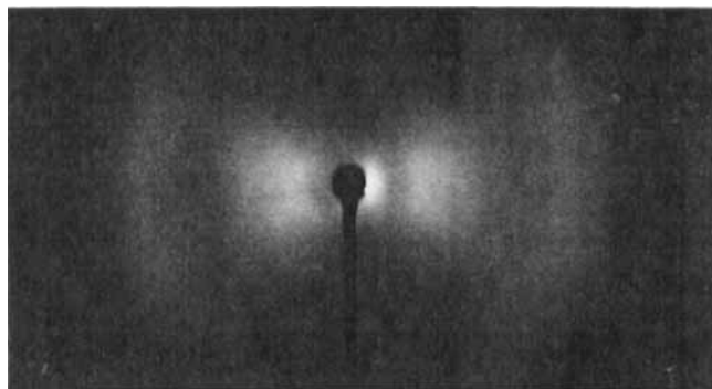
Fig. 2. AZA-9 ( n = 7 ), Polyester T_{NI} = 90^{\circ}\text{C} , \overline{M}_n = 2,000 , heated to 90^{\circ}\text{C} in a magnetic field of 10 Tesla and quenched at 73^{\circ}\text{C} to room temperature at 100^{\circ}/\text{min} . Picture is typical of n = 5, 9 and 11 .
